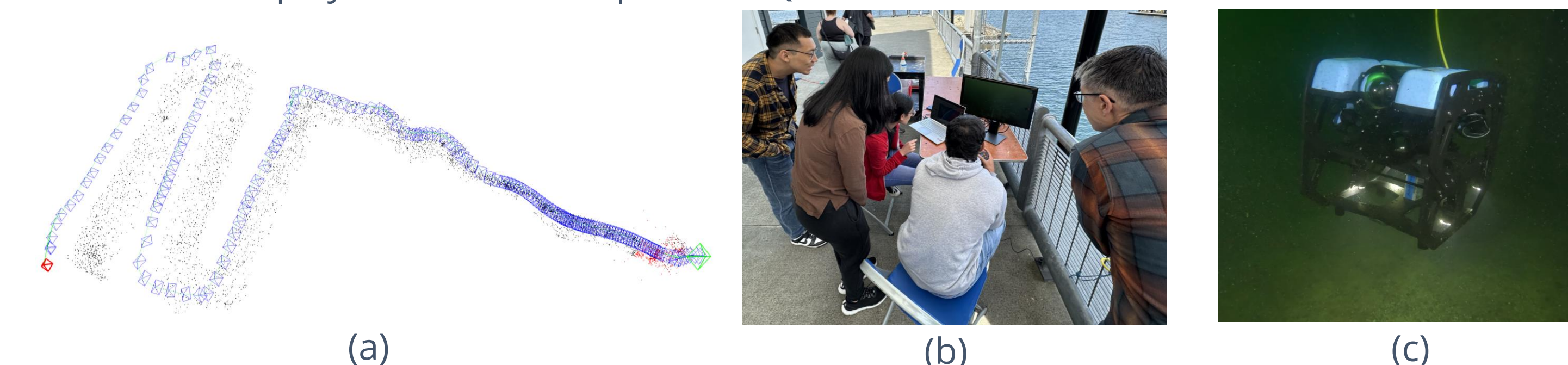
Figure 9. Test running the entire system in real-time at the pier (b and c) and the trajectory of ROV estimated by ORB-SLAM (a)
